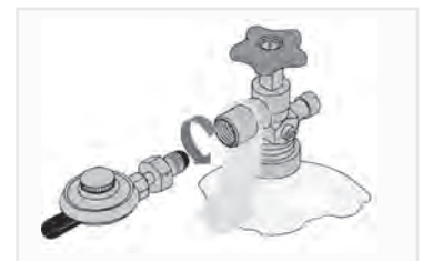
For POL cylinders, tighten anti-clockwise
