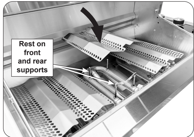
Fig. 32-2 Install flavor grids over burners
