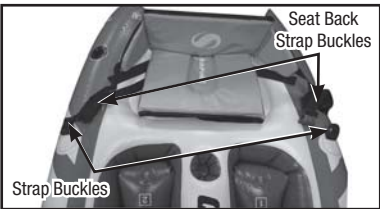
16. Connect the seat back strap buckles to the buckles on the kayak.
