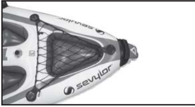
13. The cargo net installed onto kayak.
