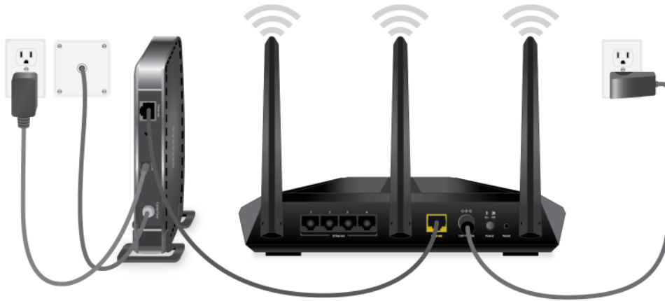
Figure 6. Cable your router
