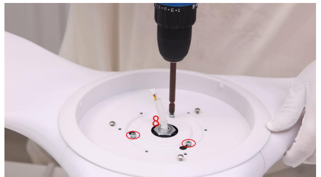
14.Tighten the 3 silver lamp panel screws
