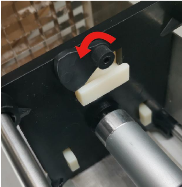
f) Pull up the top plate and remove it for replacement or cleaning
