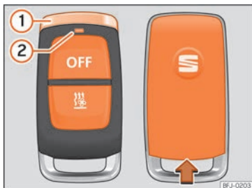
Fig. 95 Independent heating: radiofrequency remote control key
