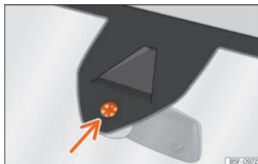
Fig. 93 Windscreen humidity and temperature sensor.
