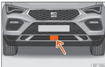
Fig. 107 On the front bumper: radar sensor.
