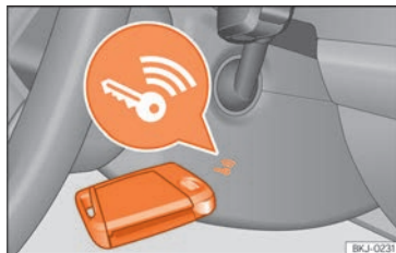
Fig. 97 On the right of the steering column: emergency start.
