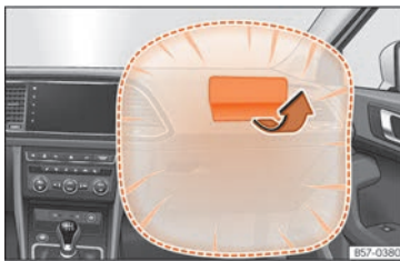
Fig. 28 Front passenger airbag located in dash panel.
