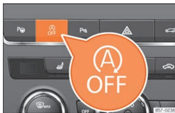
Fig. 98 Centre console: Start-Stop system button.
