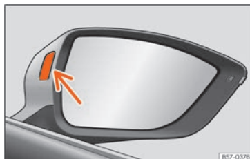
Fig. 127 Control lamp of the lane departure warning.
