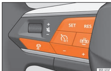
Fig. 116 On the multifunction steering wheel: buttons for operating the ACC.
