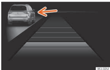
Fig. 117 On the instrument panel display: ACC active, vehicle detected on the left.
