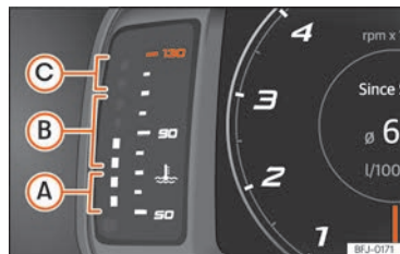
Fig. 8 SEAT Digital Cockpit digital instrument cluster: engine coolant temperature indicator.
