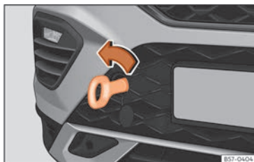
Fig. 193 Right side of the front bumper: towline anchorage screwed in.
