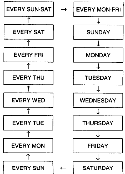
Fig. 1 Selecting the day(s) of the week When you press \Delta+ , the days of the week appear in the following order.
