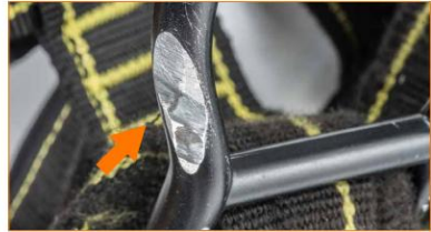
Attachment ring with clear signs of abrasion.
