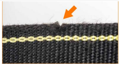
Strap with small tear on external edge.
