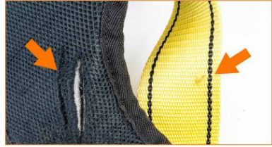
Padding damaged. Important! Check carefully any structural straps located above or below padding. You can see in the photo the slight cut mark on the right of the strap.
