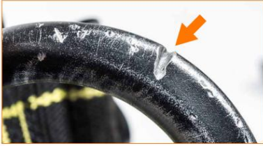
Attachment ring with cut mark.
