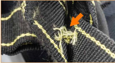
Stitches of safety stitching have been cut.
