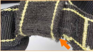
Straps very worn where they join.
