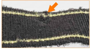
Strap with obvious loose threads.
