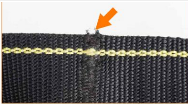
Strap has been crushed.
