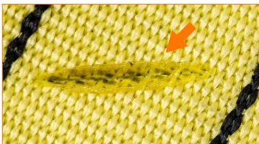
Strap has been burnt by touching hot object.
