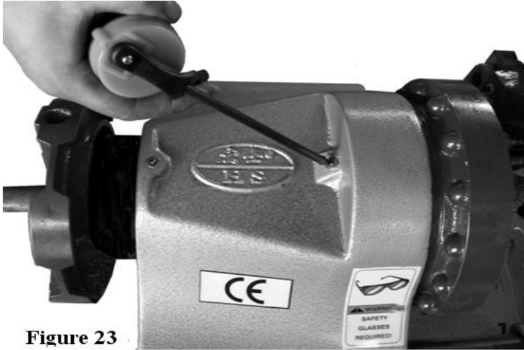
Figure 23. Location of headstock oil ports
