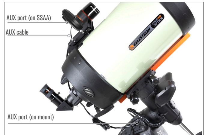
Fig. 10: Use the supplied AUX cable to connect SSAA's AUX port to the mount's AUX port.
