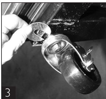
Use shims as necessary to level cabinet.
