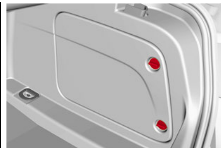
Battery Access Panel
