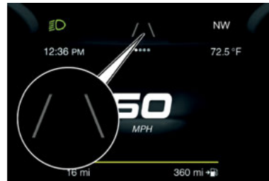
Lane Markings Not Detected
