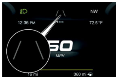
Lane Markings Not Detected
