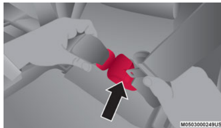
Detaching Mini-Buckle With Seat Belt Tongue
