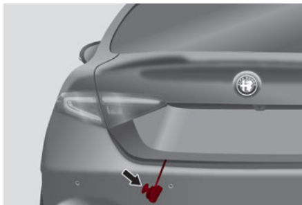
Manual Release Cord Shown With Trunk Closed
