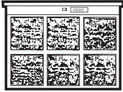
Dirty filter— Needs cleaning
