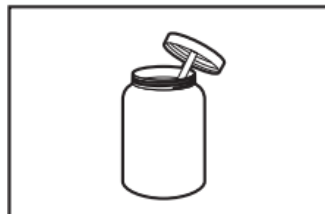
Pipe-joint compound resistant to propane gas
