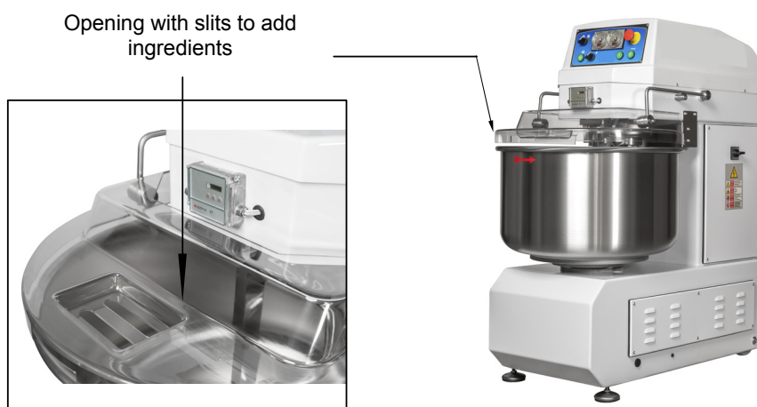
Figure 12 - Full guard: opening with slits to add ingredients
