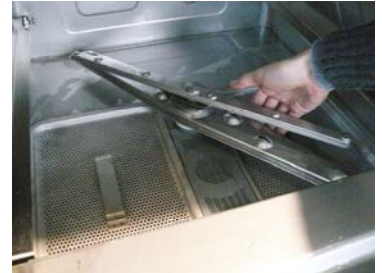
Check that the wash and rinse arms are free to rotate (upper and lower)
