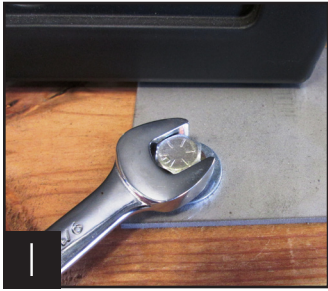
1 Removing bracket from skid.
