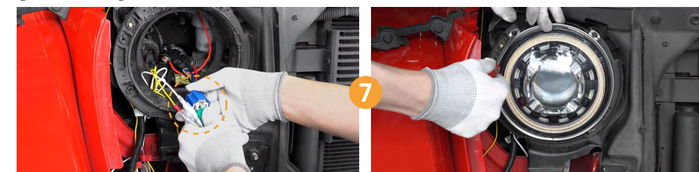
7. Now we can go ahead and plug it into the factory H4 headlight connector. Then reattach the trim ring and screws back in.
