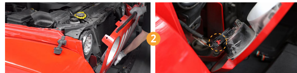
2. Remove the grille, and disconnect the turn signal connector at the bottom of the back of the grille.
