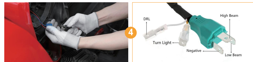
4. Disconnect the plug at the back of the factory headlight, and replace it with new headlight. Auxbeam's headlight has DRL (white wire) and turn signal (yellow wire).
