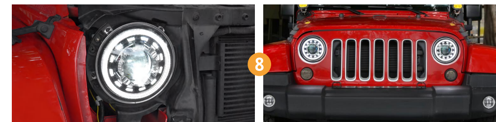
8. Repeat the steps 3-7 on the driver side, test the function of the new headlights. Once the headlights have worked properly, reinstall the grille and secure it with the original push rivets.
