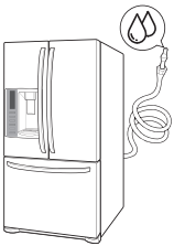
4 Connecting the water supply and water line
