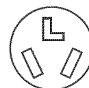
3-wire receptacle (10-30R)
