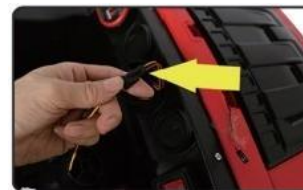
2.Insert the steering wheel control cable into the body power cord end.
