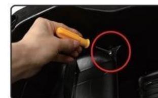
3. Align the protrusion on the back of the car with the groove on the body,buckle it into the seat,align it with the screw hole below,and tighten it with a screwdriver to fix it
