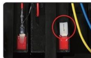
1.Remove the white insulation cap from the battery.
