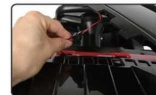
3.Insert the front windshield power cord into the body power cord end.
