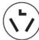
3-wire receptacle (10-30R)
