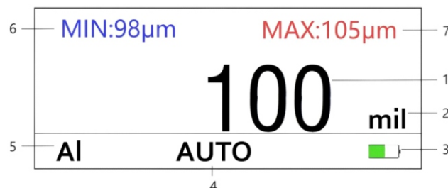
Figure 16: MIN+MAX Mode Interface Overview
