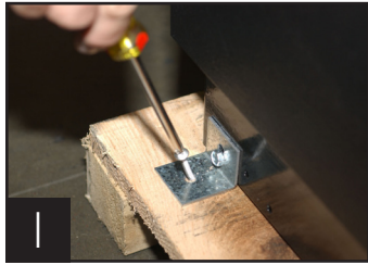
Removing bracket from skid.
