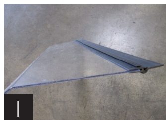
Air deflector and hinge assembly
