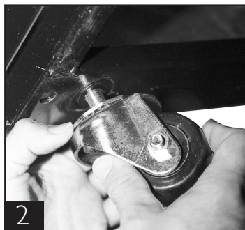
Thread castors into existing leg leveler holes.
