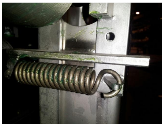
Rocker arm slip clutch spring, hook to bar weldment
