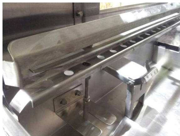
Wash tank sequence bar, pendulum with magnet
