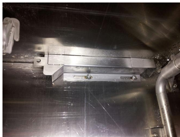
Diverter plate separates fill stream for wash and rinse tank
