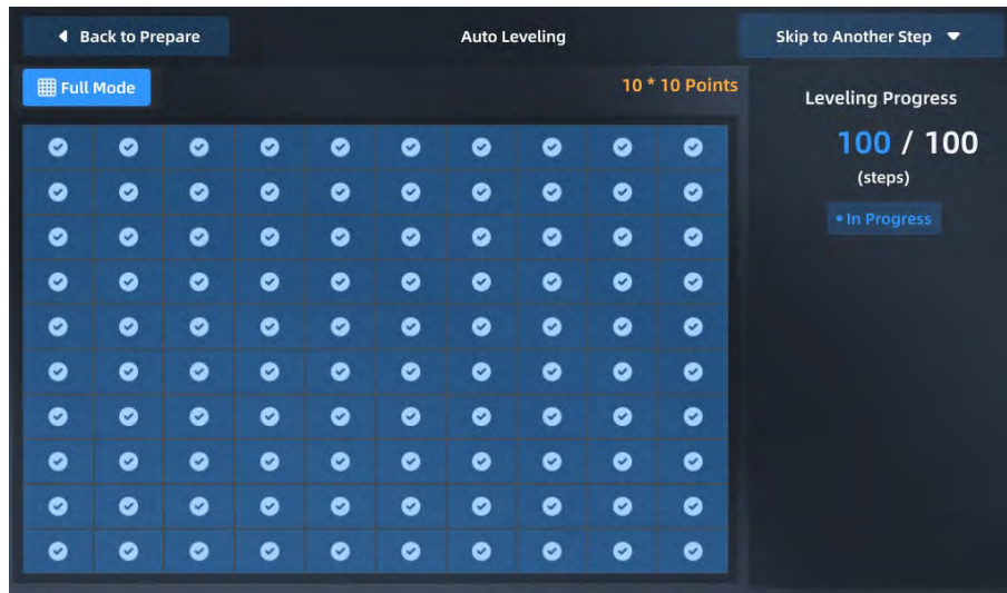
Fig. 4.48 Completion of 100-Point Leveling
