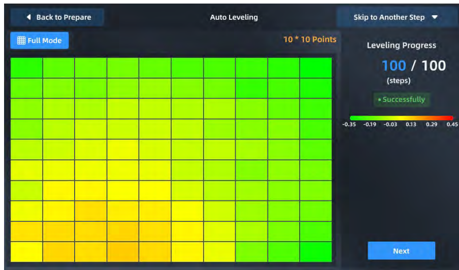
Fig. 4.49 100-Point Leveling Successful
