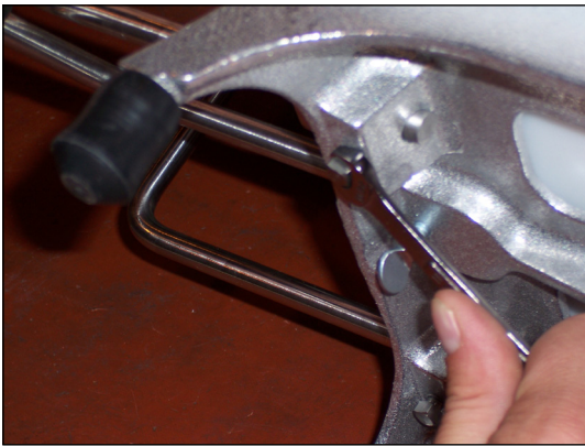
Figure 4. Pusher Head Adjustment Through the Blades.
