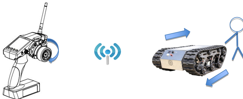
Steering mix throttle setup completed, left track moves forward while right backward when turning the wheel clockwise. The differential realizes the right turning of track vehicle
