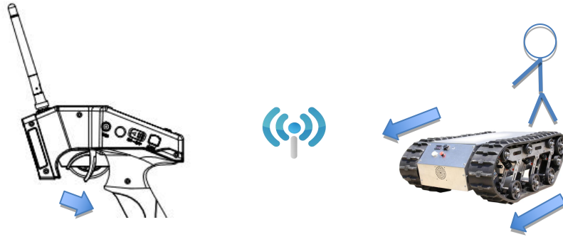
Throttle mix steering setup completed, both tracks moves forward when pulling the throttle
