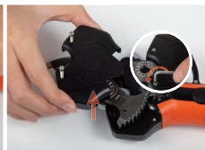
4. Loosen the cap's screw and remove the cap.
