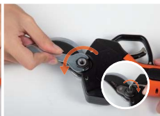
2. Loosen the small locking nut in a clockwise direction, and take off the stop washer. Loosen the big locking nut in an anticlockwise direction.
