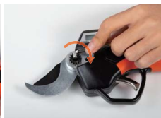
3. Loosen the big screw with wrench in a clockwise direction.
