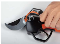
1. Loosen the small screw with wrench in an anticlockwise direction.
