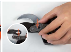
8. Install the upper blade and swing gear.
