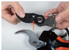
5. Remove the upper blade and swing gear.
