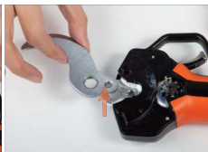
6. Remove the lower blade.
