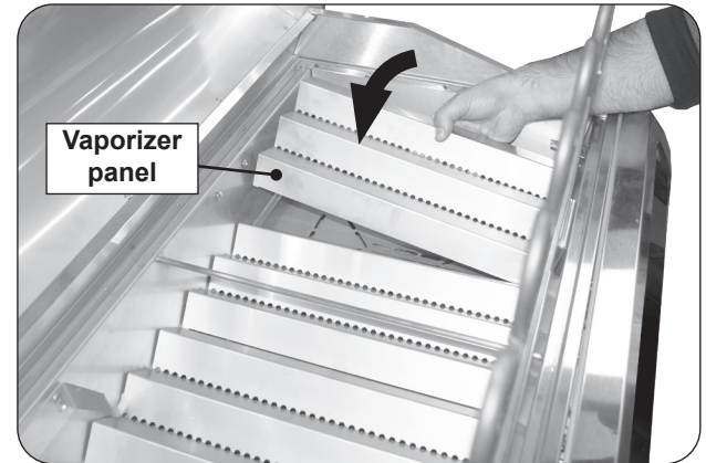
Fig. 34-2 Install vaporizer panels
