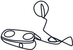
Red emergency stop magnet
