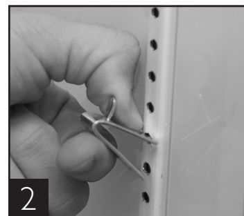
Installing bottom of the shelf clip
