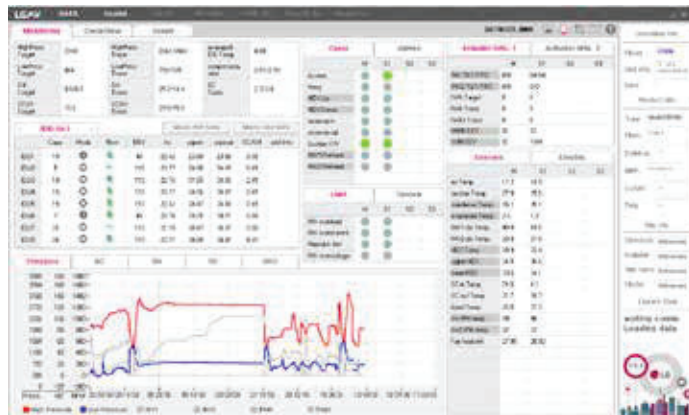
Figure 131: LGMV Monitoring Screen.
