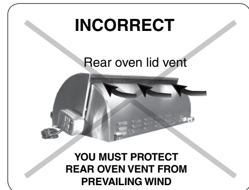
Fig. 12-3 Airflow direction - INCORRECT
