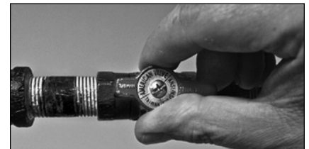
Figure 51 - Gas valve in “on” position.
