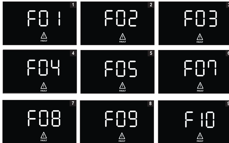
Figure 16. Critical Fault Screens
