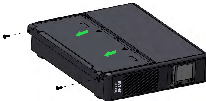
Figure 76. Battery Cover Removal
