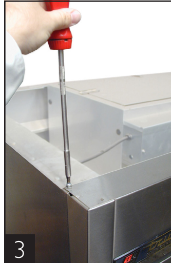
Rainshield removal, top screws.
