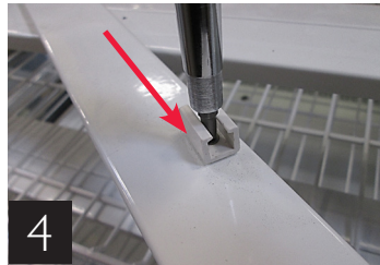
3 Press shelf into retainer
