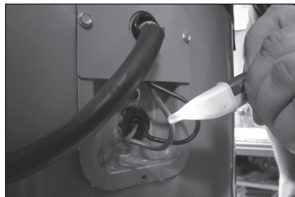
Figure 43 - Non-Contact Circuit Tester.
