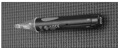
Figure 32 - Use a non-contact circuit tester to check for electrical power.
