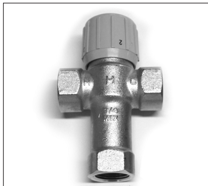
Figure 8 - Thermostatic Mixing Valves installed at each point-of-use can help prevent scalds.
