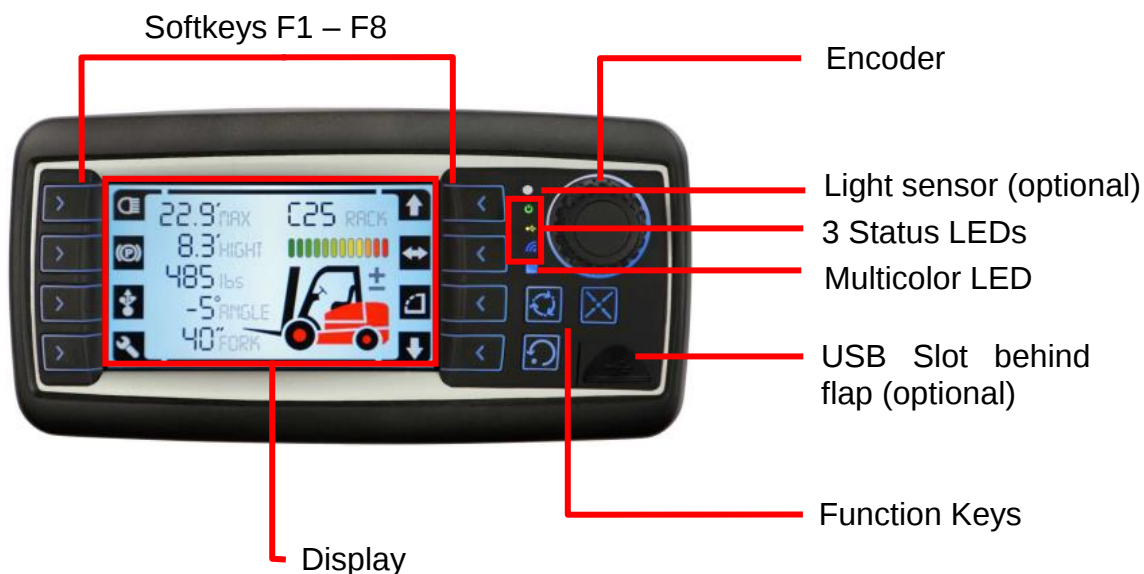
Fig. 3.2: Schematic diagram of the OPUS A3 STANDARD Landscape
