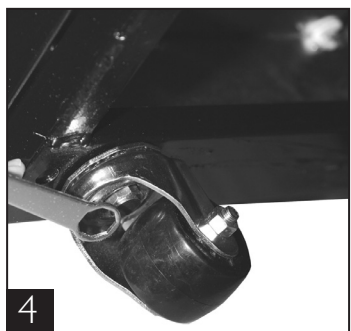
Tighten castor in position with castor wrench.
