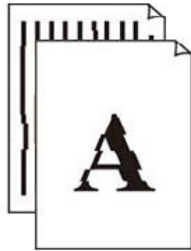
Lines Are Misaligned/Distorted
