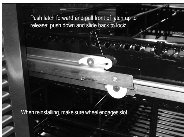
Figure 16: Removing/Installing Drawer
