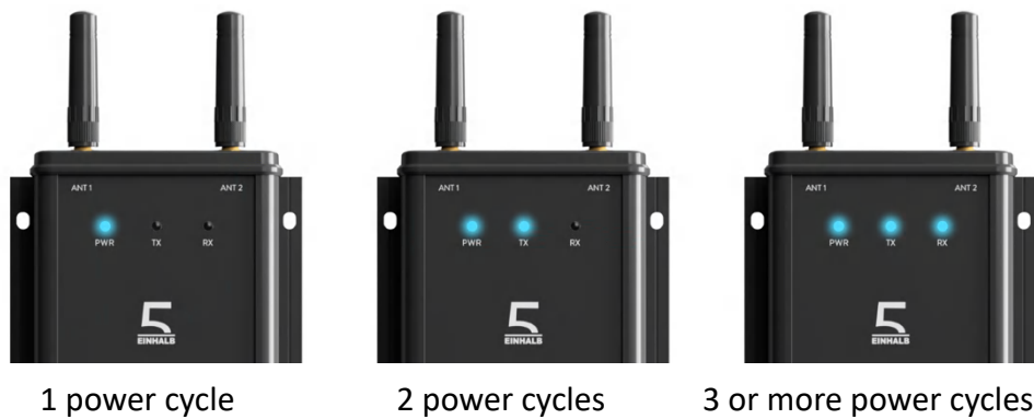
Figure 12 Visualization of how the device displays the number of power cycles performed at the beginning of its startup phase. This also applies to access points.
