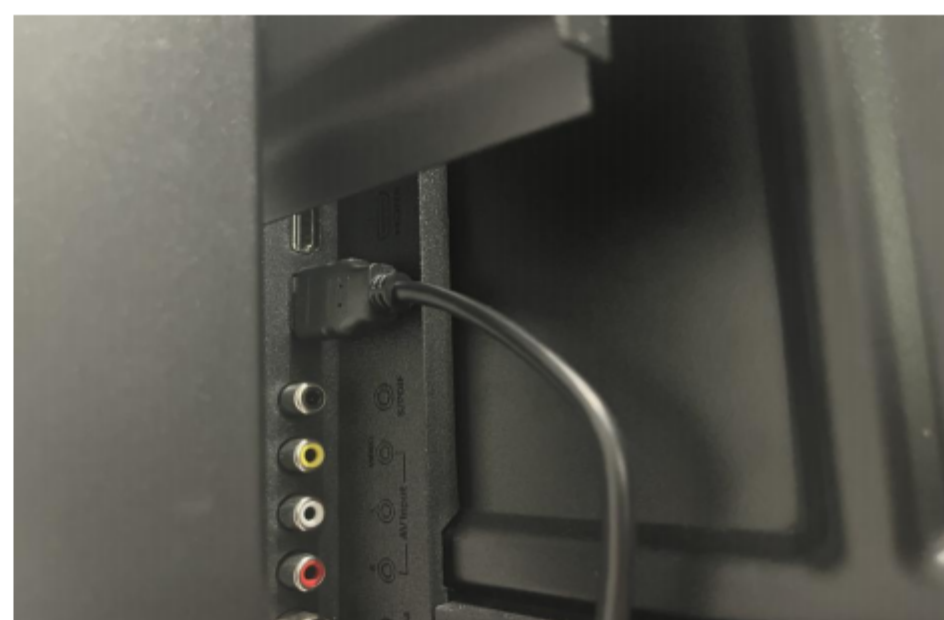
The picture shows the connection between HDMI extension adapter and TV
