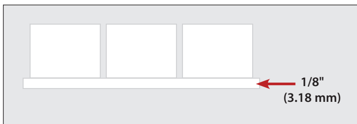
Fig. 1. The ice bridge holds the ice cubes together.
