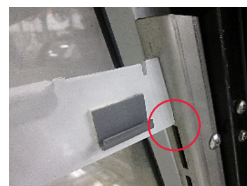
Bottom notch installed (no gap)
