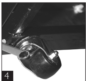
Tighten castor in position with castor wrench.
