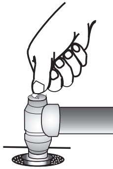
Figure 6. Testing the Temperature-Pressure Relief Valve
